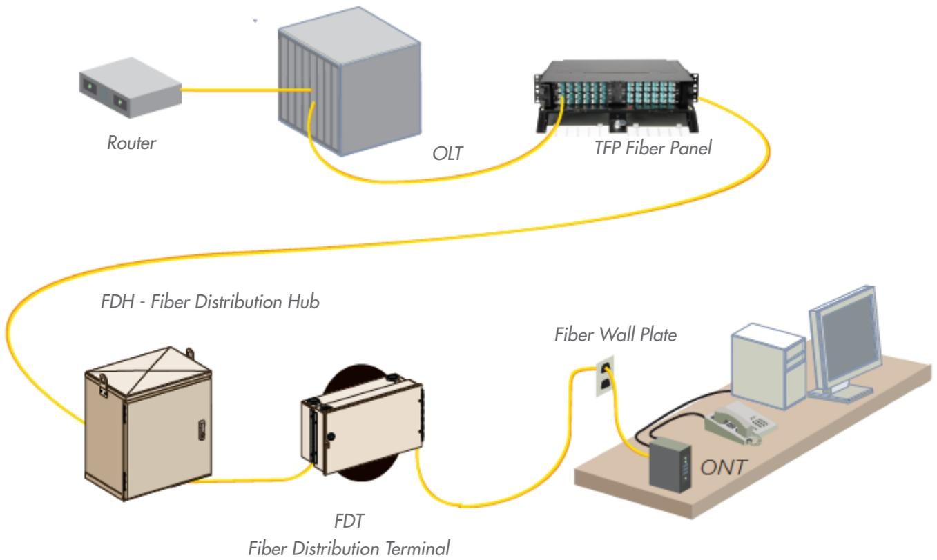
TIA headquarters features a PON design using CommScope's OLS which takes up less floor space and requires less cable.
