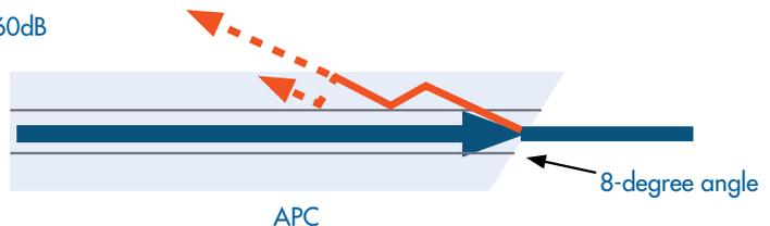
The flat connector interface of a UPC connector reflects light back at the source, while the angle of the APC connector reflects the light into the cladding.
