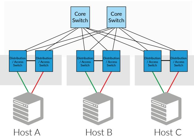
Figure 2: This illustrates a collapsed two-tier network.
