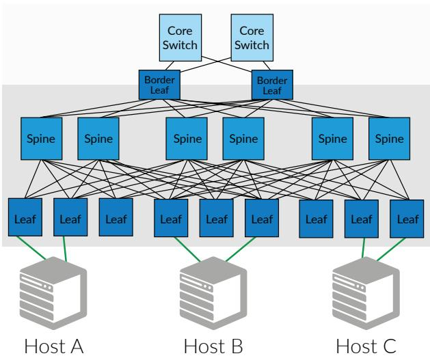
Figure 3: The IT industry is now deploying cloud-friendly leaf-spine networks.
