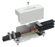
Cable unit break out kit for low fiber count loose tube cables (max 24mm), 1 cable to max 6 flex tubes (ID 6mm). Cable application range subject of loose tube diameter and stiffness (indicatively: max 288f cable with 1,7 mm loose tube)
