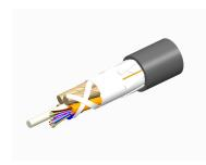
Fiber indoor/outdoor cable, LazrSPEED®, Single Jacket All-Dielectric, Plenum Rated, Gel-Free, Stranded Loose Tube, PVDF jacket, 96 fiber, Multimode OM3, Black jacket color, Feet cable marking
