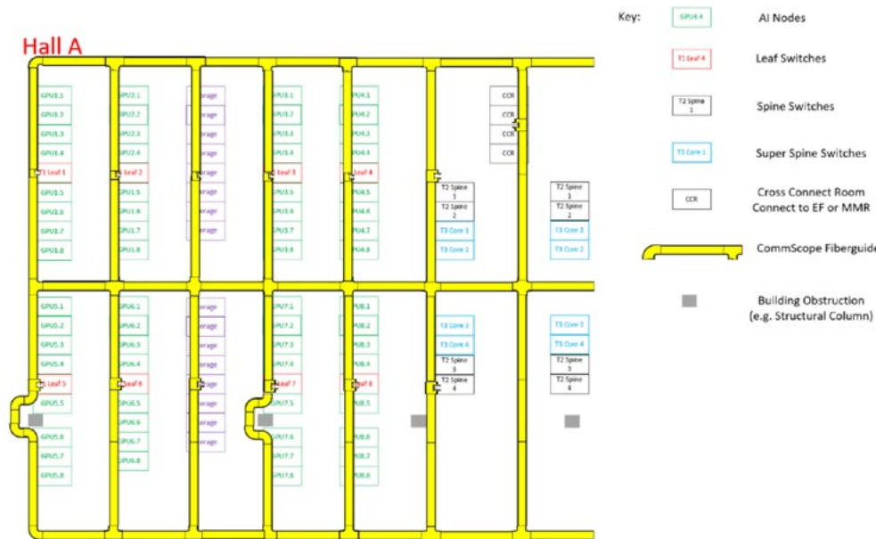
Figure 1 - Example Gen DC AI layout using the FiberGuide system. The switching layers have more physical separation than traditional designs, allowing for the power and cooling constraints of a traditional data center construction.
