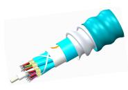
Fiber indoor cable, TeraSPEED® Low Smoke Zero Halogen Riser Distribution, interlocking aluminum armored, Multimode/Singlemode, 48 fiber multi-unit with 12 fiber subunits, Gel-free, Feet jacket marking, Aqua jacket color, B2ca flame rating
