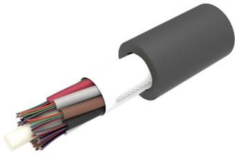
Fiber indoor/outdoor cable, Low Smoke Zero Halogen, 96 fiber Microsheath, Multi mode OM4 , Gel-free, Meters jacket marking, Black jacket color, B2ca flame rating
