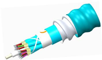
LazrSPEED® Plenum Distribution Cable, interlocking aluminum armored with plenum jacket, 96 fiber multi-unit with 12 fiber subunits
