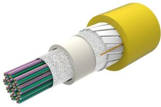
Fiber indoor cable, All-Dielectric, Riser-Rated, Gel-Free, Central Tube with 12x200um Rollable Ribbons, 1728 fiber, G.652.D / G.657.A1 Singlemode , Feet jacket marking, Yellow jacket color
