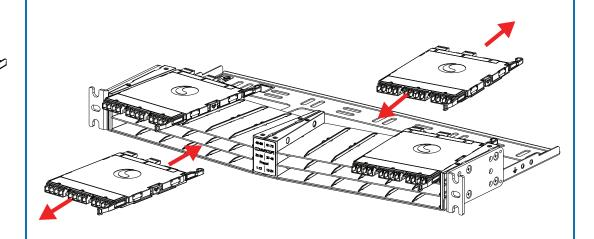
**b** Align grooves on bottom of adapter pack or module with rails on blade. Slide in on rails.
