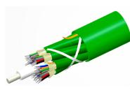
Fiber indoor cable, TeraSPEED® Plenum Distribution, 72 fiber multi-unit with 12 fiber subunits, Singlemode G.652.D and G.657.A1, Gel-free, Feet jacket marking, Green jacket color
