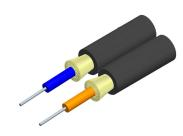
Fiber indoor/outdoor cable, TeraSPEED® 1.6 mm Low Smoke Zero Halogen Riser Zipcord 2-fiber, Singlemode G.652.D and G.657.A1, Gelfree, Feet jacket marking, Black jacket color
