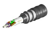
Fiber indoor/outdoor cable, TeraSPEED®, Plenum Rated, 120 fiber, Singlemode G.652.D and G.657.A1, Gel-Free, Stranded Loose Tube with Aluminum Interlocking Armor containing a Plenum Rated Outer Jacket, Black jacket color, Feet cable marking
