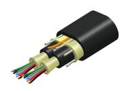
Fiber Indoor/Outdoor cable, TeraSPEED® Low Smoke Zero Halogen Riser MPO Trunk, 24 fiber with 12 fiber subunits, Gel-free, Singlemode G. 652.D and G.657.A1, Feet jacket marking, Black jacket color, Dca flame rating
