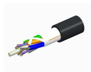
Fiber indoor/outdoor cable, TeraSPEED®, Single Jacket All-Dielectric (LSZH), 12 fiber, Singlemode G.652.D and G.657.A1, Gel-Free, Stranded Loose Tube, Black jacket color, Feet cable marking, Eca flame rating
