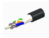
Fiber indoor/outdoor cable, LazrSPEED®, Single Jacket All-Dielectric, Low Smoke Zero Halogen (LSZH), Gel-Free, Stranded Loose Tube, 12 fiber, Multimode OM3, Black jacket color, Feet cable marking, Eca flame rating
