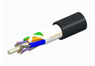
Fiber indoor/outdoor cable, LazrSPEED®, Single Jacket All-Dielectric, Low Smoke Zero Halogen (LSZH), 24 fiber, Gel-Free, Stranded Loose Tube, Multimode OM3, Black jacket color, Feet cable marking, Eca flame rating
