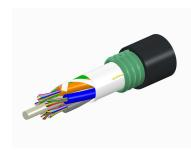
Fiber indoor/outdoor cable, TeraSPEED®, Single Jacket/Single Armor, Low Smoke Zero Halogen (LSZH), 6 fiber, Singlemode G.652.D and G. 657.A1, Gel-Free, Stranded Loose Tube, Black jacket color, Feet jacket marking
