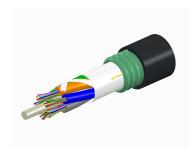
Fiber indoor/outdoor cable, TeraSPEED®, Single Jacket/Single Armor, Low Smoke Zero Halogen (LSZH), 12 fiber, Singlemode G.652.D and G. 657.A1, Gel-Free, Stranded Loose Tube, Black jacket color, Feet jacket marking
