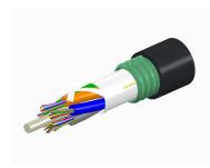
Fiber indoor/outdoor cable, TeraSPEED®, Single Jacket/Single Armor, Low Smoke Zero Halogen (LSZH), 24 fiber, Singlemode G.652.D and G. 657.A1, Gel-Free, Stranded Loose Tube, Black jacket color, Feet jacket marking
