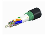
Fiber indoor/outdoor cable, TeraSPEED®, Single Jacket/Single Armor, Low Smoke Zero Halogen (LSZH), 36 fiber, Singlemode G.652.D and G. 657.A1, Gel-Free, Stranded Loose Tube, Black jacket color, Feet jacket marking
