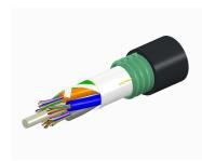
Fiber indoor/outdoor cable, TeraSPEED®, Single Jacket/Single Armor, Low Smoke Zero Halogen (LSZH), 48 fiber, Singlemode G.652.D and G. 657.A1, Gel-Free, Stranded Loose Tube, Black jacket color, Feet jacket marking
