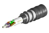
Fiber indoor/outdoor cable, LazrSPEED®, Plenum Rated, Multimode OM4, 72 fiber, Gel-Free, Stranded Loose Tube with Aluminum Interlocking Armor jacket, Gel-free, Feet jacket marking, Black jacket color
