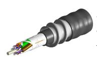
Fiber indoor/outdoor cable, LazrSPEED®, Plenum Rated, Gel-Free, 24 fiber, Stranded Loose Tube with Aluminum Interlocking Armor containing a Plenum Rated Outer Jacket, Multimode OM3, Feet jacket marking, Black jacket color
