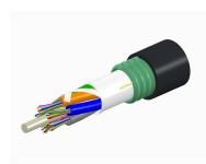
Fiber OSP cable, TeraSPEED® Single Jacket/Single Armor, Gel-Free, 96 fiber, Stranded Loose Tube, Composite OM4 and G.652.D and G.657.Al, Feet jacket marking, Black jacket color
