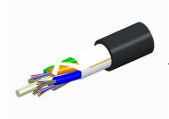
Fiber OSP cable, TeraSPEED® Single Jacket All-Dielectric, 168 fiber, Gel-Free, Stranded Loose Tube, Singlemode G.652.D and G.657.A1, Feet jacket marking, Black jacket color
