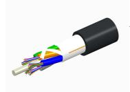
Fiber OSP cable, TeraSPEED® Single Jacket All-Dielectric, Gel-Free, 96 fiber, Stranded Loose Tube, Composite OM3 and G.652.D and G.657.A1, Feet jacket marking, Black jacket color
