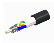
Fiber OSP cable, TeraSPEED® Single Jacket All-Dielectric, Gel-Free, 96 fiber, Stranded Loose Tube, Composite OM3 and G.652.D and G.657.Al, Feet jacket marking, Black jacket color
