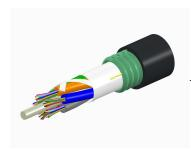
Fiber OSP cable, TeraSPEED® Single Jacket/Single Armor, 132 fiber, Gel-Free, Stranded Loose Tube, Singlemode G.652.D and G.657.A1, Feet jacket marking, Black jacket color
