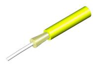
Fiber Indoor Cable, TeraSPEED® 2.9mm Low Smoke Zero Halogen Riser, 1-fiber Simplex, Singlemode G.652.D and G.657.A1, Feet jacket marking, Yellow jacket color
