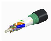
Fiber OSP cable, TeraSPEED® Single Jacket/Single Armor, Gel-Free, 6 fibers, Stranded Loose Tube, Singlemode G.652.D and G.657.A1, Feet jacket marking, Black jacket color
