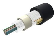
Fiber indoor/outdoor Cable, LSZH Riser All-Dielectric Central Tube Ribbon, Multimode OM3 bend insensitive, 192-fiber, feet jacket marking, black jacket color
