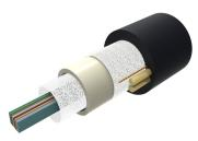
Fiber OSP Cable, Non-Armored, All-Dielectric, Arid-Core, 96 fiber, Dry Central Tube Ribbon, Singlemode G.652.D and G.657.Al, Gel-free, Feet jacket marking, Black jacket color
