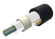
Fiber OSP Cable, Non-Armored, All-Dielectric, 144 fiber, Arid-Core, Dry Central Tube Ribbon, Singlemode G.652.D and G.657.Al, Gel-free, Feet jacket marking, Black jacket color
