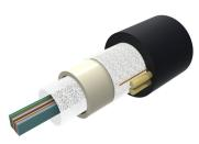
Fiber OSP Cable, Non-Armored, All-Dielectric, Arid-Core, 360 fiber, Dry Central Tube Ribbon, Singlemode G.652.D and G.657.Al, Gel-free, Feet jacket marking, Black jacket color
