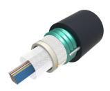
Fiber OSP cable, Steel Armored, Arid-Core, Dry Central Tube Ribbon, 144 fiber, Singlemode G.652.D and G.657.A1, Feet jacket marking, Black jacket color
