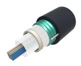
Fiber OSP cable, Steel Armored, Arid-Core, Dry Central Tube Ribbon, 432 fiber, Singlemode G.652.D and G.657.A1, Feet jacket marking, Black jacket color
