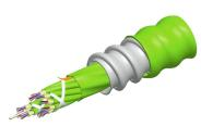
Fiber indoor cable, LazrSPEED® Riser Distribution, interlocking aluminum armored with riser jacket, 96 fiber multi-unit with 12 fiber subunits, Multimode OM5, Feet jacket marking, Lime green jacket marking
