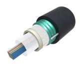
Fiber OSP cable, Steel Armored, Arid-Core, Dry Central Tube Ribbon, 576 fiber, Singlemode G.652.D and G.657.A1, Feet jacket marking, Black jacket color
