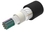
Fiber indoor/outdoor cable, All-Dielectric, LSZH Riser-Rated, Gel-Free, Central Tube Rollable Ribbon, 576 fiber, Singlemode G.652.D and G.657. Al, Feet jacket marking, Black jacket color, Cca flame rating
