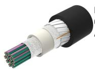
Fiber indoor/outdoor cable, All-Dielectric, LSZH Riser-Rated, Gel-Free, Central Tube Rollable Ribbon, 864 fiber, Singlemode G.652.D and G.657. Al, Feet jacket marking, Black jacket color, Cca flame rating
