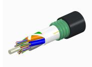
Fiber indoor/outdoor cable, LazrSPEED®, Single Jacket/Single Armor, Low Smoke Zero Halogen (LSZH), 24 fiber, Multimode OM4, Gel Filled , Stranded Loose Tube, Black jacket color, Meters jacket marking, Cca flame rating
