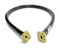
FlexTwist® Flexible Twist for WR90, 8.2–12.4 GHz, with interface types PDR100 and PBR100, 600 mm
