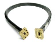
FlexTwist® Flexible Twist for WR187, 4.4–5.0 GHz, with interface types PDR48 and UDR48, 300 mm
