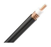
AVA5RK-50FX, HELIAX® Andrew Virtual Air™ Coaxial Cable, corrugated copper, 7/8 in, black, Non-halogenated, fire retardant polyolefin jacket B2ca-sl, d2,al (CPR testing is conducted annually please reference the website for latest classification)
