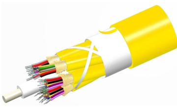
Fiber indoor cable, TeraSPEED® Low Smoke Zero Halogen Riser Distribution, 72 fiber multi-unit with 12 fiber subunits, Gel-free, Singlemode G.652.D and G.657.A1, Feet jacket marking, Yellow jacket color
