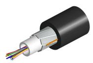
Fiber Indoor/Outdoor Drop Cable, TeraSPEED®, Low Smoke Zero Halogen Single Jacket All-Dielectric Arid-Core, 2-fiber, Gel-filled, Singlemode G.652.D and G.657.A1, Feet jacket marking, Black jacket color, Dca flame rating
