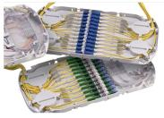
FIST GPST Fiber Patch/Splice Tray, 24 ports, LC/APC, singlemode, preterminated with pigtails, SMOUV splice chip, 19 in, gray, left patch cord routing
