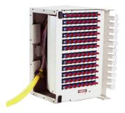
OMX Fiber Termination Block, pre-terminated with pigtails, 96 SC/UPC, singlemode, putty white, right oriented
