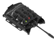
Fiber Indexing Terminal, 1x8 Splitter, 4x3 Port Design, 8 Forward Ports, 1 Reverse Port, Dielectric Flat Loose Tube Cable, 1500 Feet
